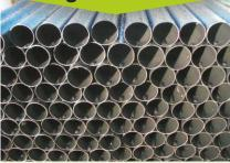
Low pressure pipes and irrigation tubes can be manufactured from medium, low, and high density, virgin or reprocessed polyethylene up to 250mm OD to industry standard dimensional specifications such as SDR11, SDR17.6 and SDR26. Other specific wall thickness' can be achieved as required. These tubes can be supplied in coils up to 110mm OD. Larger sizes can be supplied in straight lengths up to 12m. Dewatering tubes can be supplied to your exact dimensional specification.
