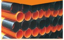
A range of smooth bore solid wall polyethylene ducting that meets the industry standard dimensional requirements. OD's, colours, wall thickness' and lengths offered as required. Black marked "Electric Cable Duct" Orange "Street Lighting" & "Traffic Signal" Purple "Spare Comms" & "Motorway Communications" other colours such as green are also available. All supplied with easy fit couplings.
